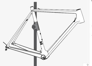
**NOTICE** Irreparable damage to the frame tube (crushing) as a result of unsuitable clamping by mounting stands.
