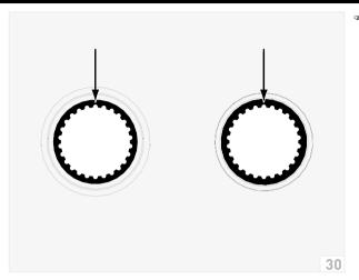
Apply a light coat of grease to the inner teeth of the hub and rotor. [fig. 30]
