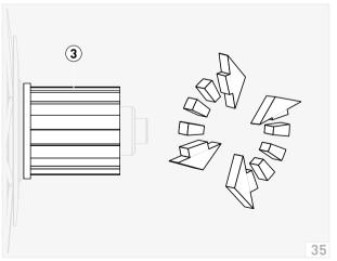
Check the function of the freewheel mechanism by turning the rotor (3) jerkily and alternately in both directions. (fig. 35)
