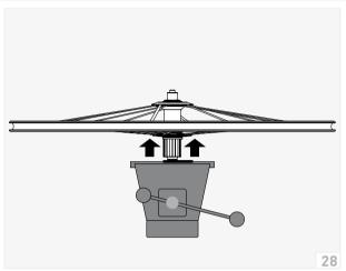
Clamp the rear whe el adapter of the rotor side in a vice using an appropriate axle retainer.
