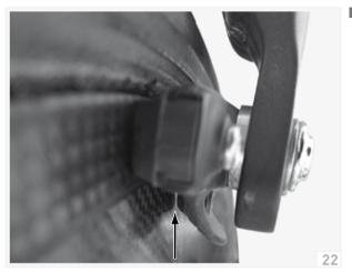
WOTICE AUTOBAHN & FERNWECT Brake shoes on race bikes are generally fitted with a "wing". It is used as an guide during installation of the wheel. (fig. 22) Because of the aerodynamic rim profile of Lightweight Aero wheels, the wing may come into contact with the surface of the rims when the brake pad is 50% worn.
