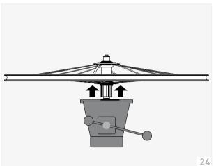
Clamp the limit stop of the rotor side in a vice using an appropriate axle retainer.
