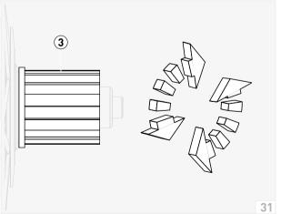
① Check the function of the freewheel mechanism by turning the rotor [3] jerkily and alternately in both directions. [fig. 31]
