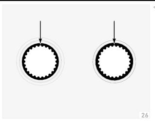
Apply a light coat of grease to the inner teeth of the hub and rotor. (fig. 26)
